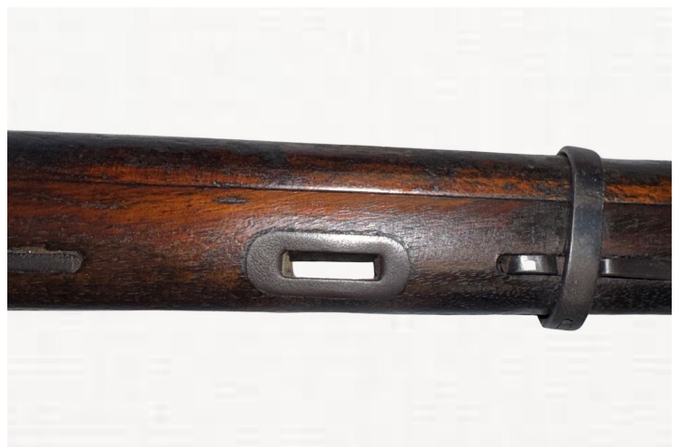
Slots for rifle sling attachment, on the forestock.
