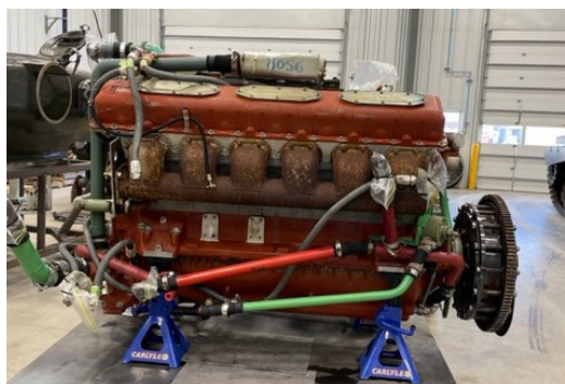
V12 out of M36 Tank.
