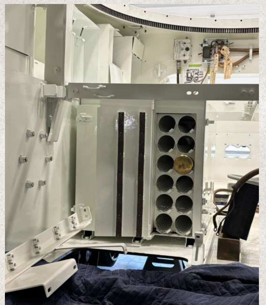
Interior of the M4A2 Sherman hull showing the wet storage ammo racks.
